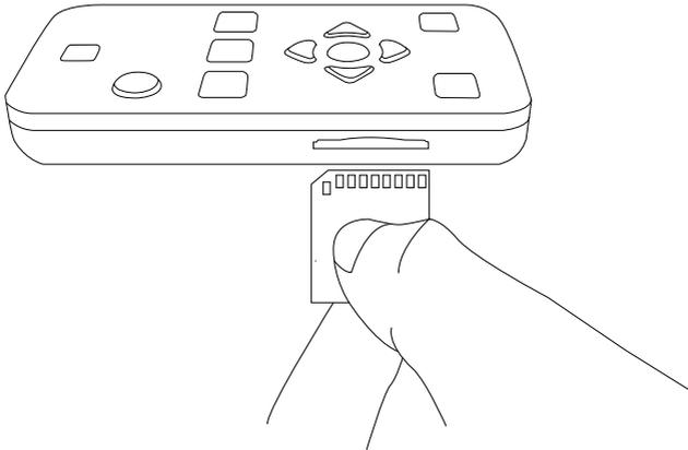
To remove the SD card, gently press the SD card into the card slot until it clicks, then release it. The SD card will pop out of the slot enough for you to grip it and pull it out completely. If the Blaze EZ is turned on, you will hear a sound to confirm that it has detected the removal of the SD card.
